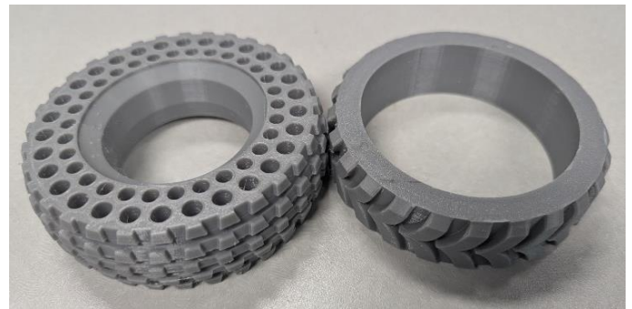
Fig. 2: Examples of 3D printed wheel design, CAVS MSU
