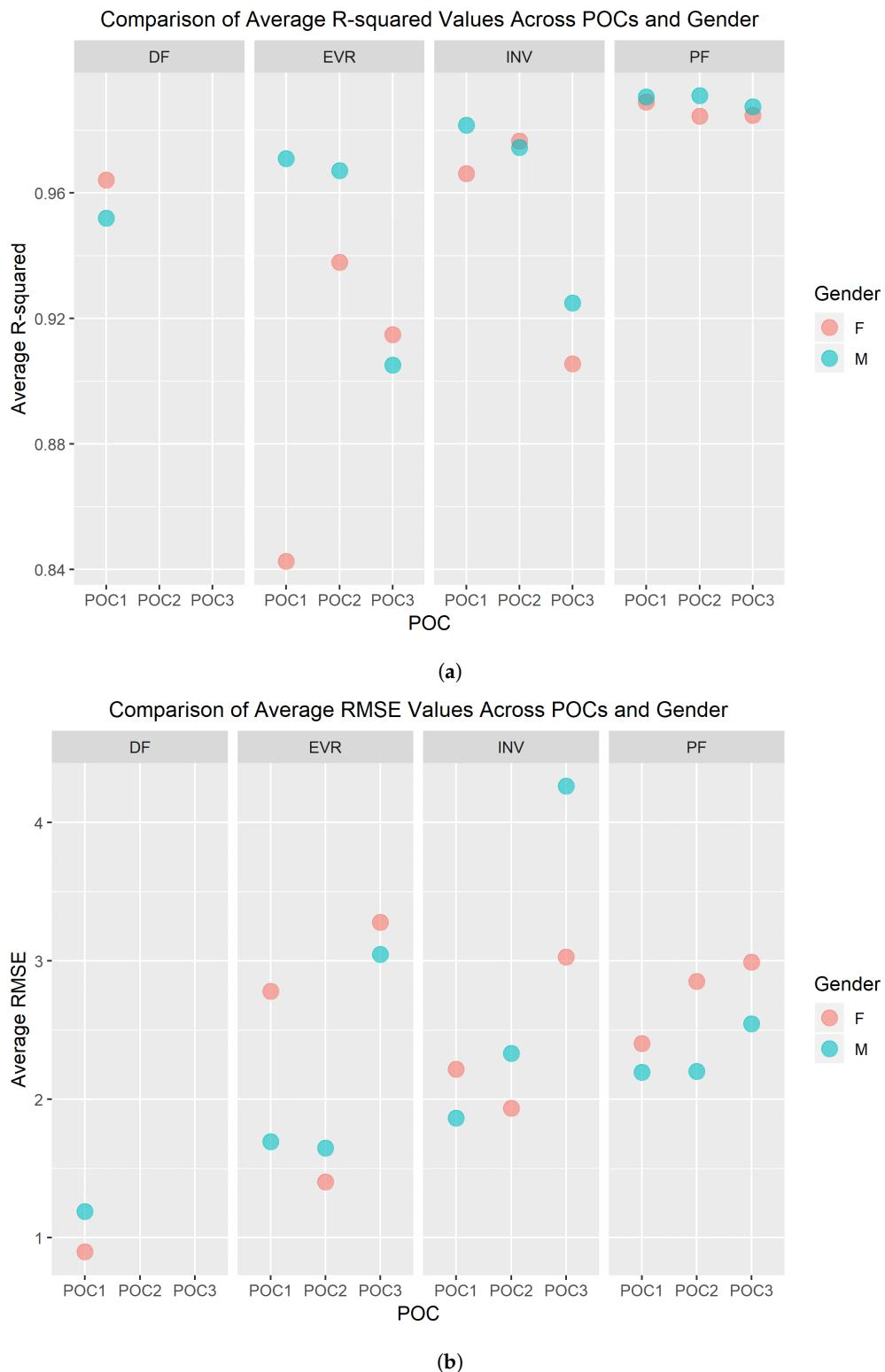
**Figure 12.** (a) Comparison of average  $R^2$  values for all SRS between genders/foot size; and (b) comparison of average RMSE values for all SRS between genders/foot size.
