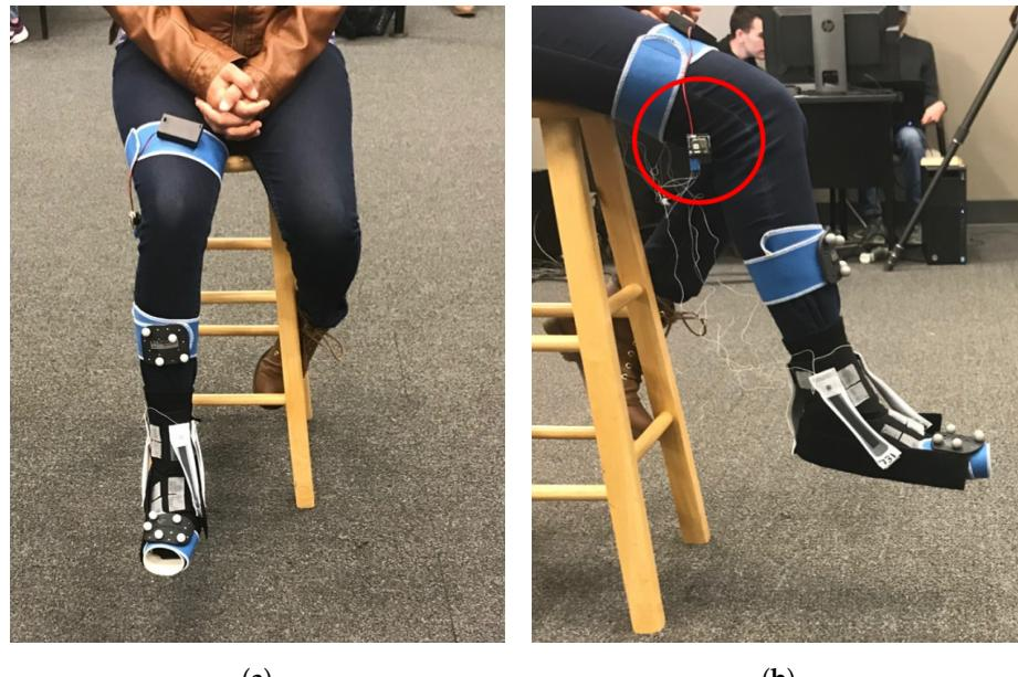
**Figure 6.** Participant image showing SRS and motion capture sensors: (a) front view; and (b) side view. The SRS sensing module is circled in red.
