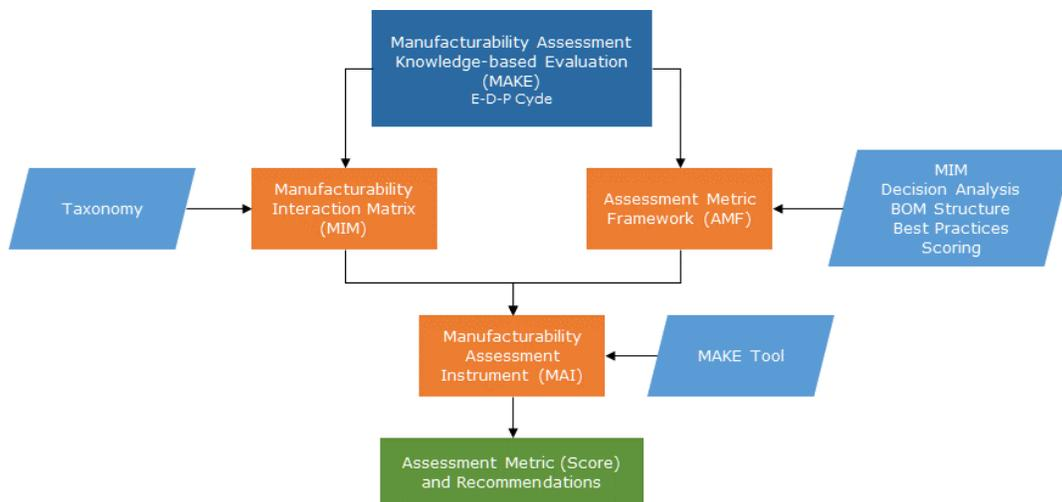
**The Manufacturability Interaction Matrix (MIM).** The MIM is a taxonomy-based system used to classify the key criteria of manufacturability. The matrix serves as the basis for the assessment and is used to provide a structured process for evaluating parts and assemblies within a given design.
