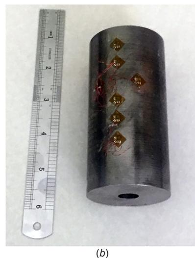
Fig. 12 (a) Hoop strain contours on the cylindrical die after simulated compaction of a FC-0205 copper steel powder and (b) strain gauges located on cylindrical die to measure hoop strain during compaction of FC-0205 powder
