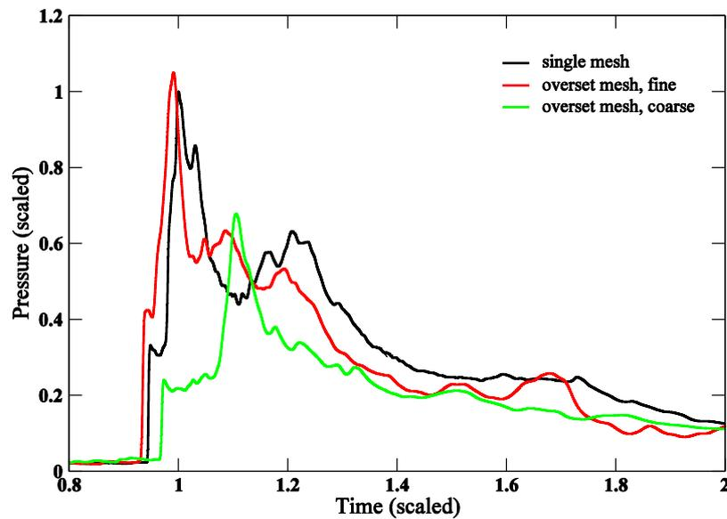
**Figure 2. Comparison of resolved blast waves on different meshes**
