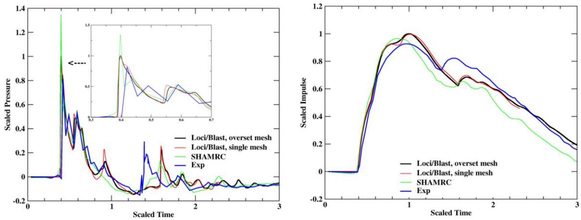
Figure 7. History of pressure (left) and impulse (right) of probe T, small building only
