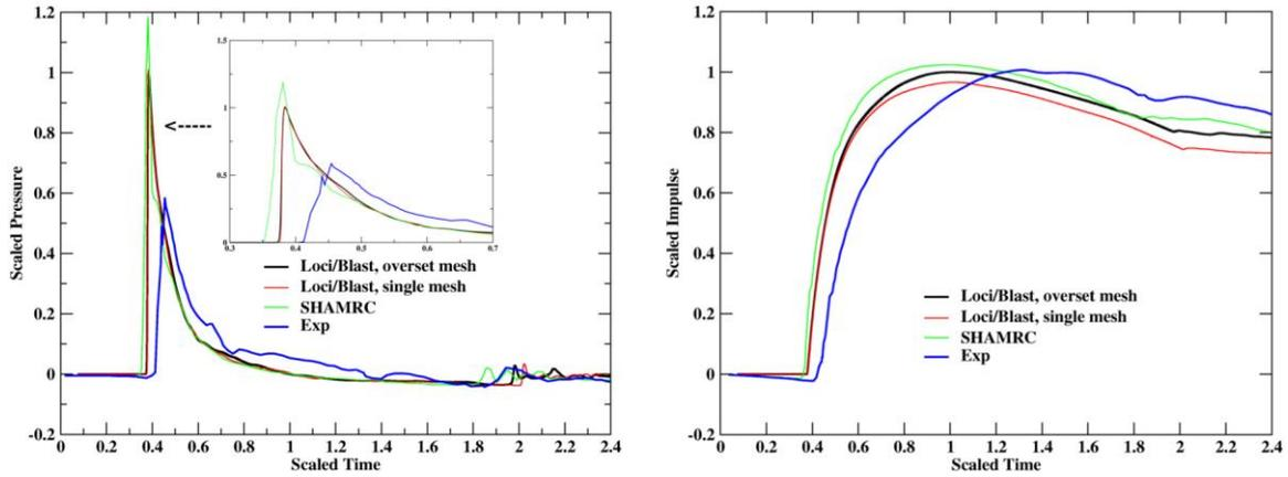
Figure 6. History of pressure (left) and impulse (right) of probe S, small building only
