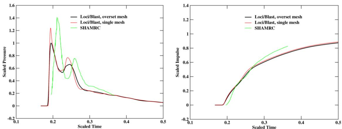
**Figure 5. History of pressure (left) and impulse (right) at probe F, small building only**
