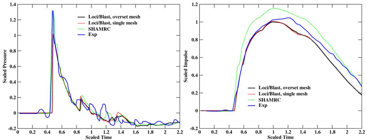
Figure 8. History of pressure (left) and impulse (right) of probe B, small building only
