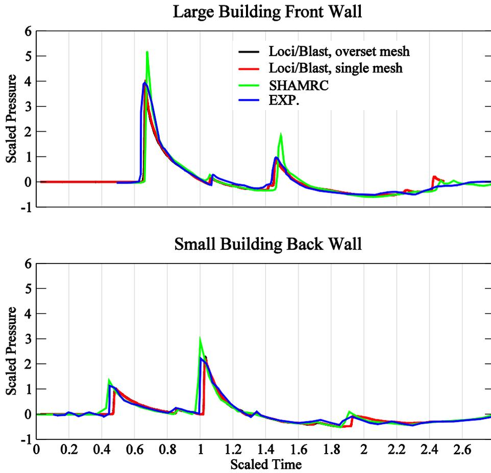
Figure 9. Alternating occurrence of pressure peaks due to wave reflections between large building (top) and small building (bottom)
