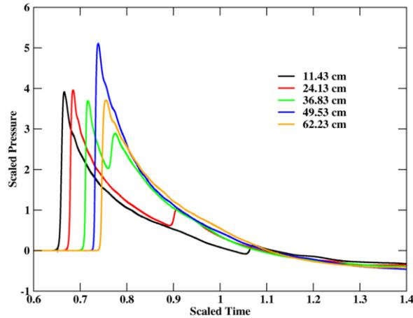
**Figure 13. Pressure peak moving up (identified by height) along the front wall of the large building**
