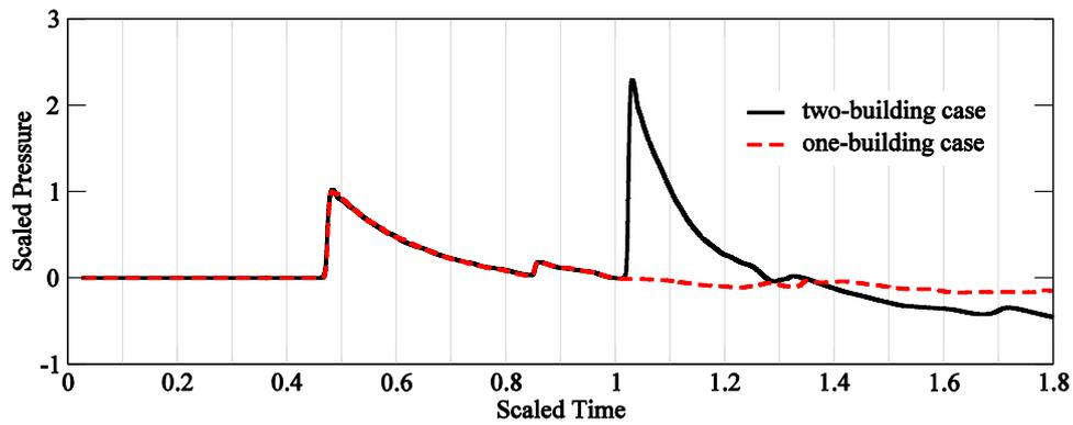
Figure 10. Predicted pressures for the back of the small structure.
