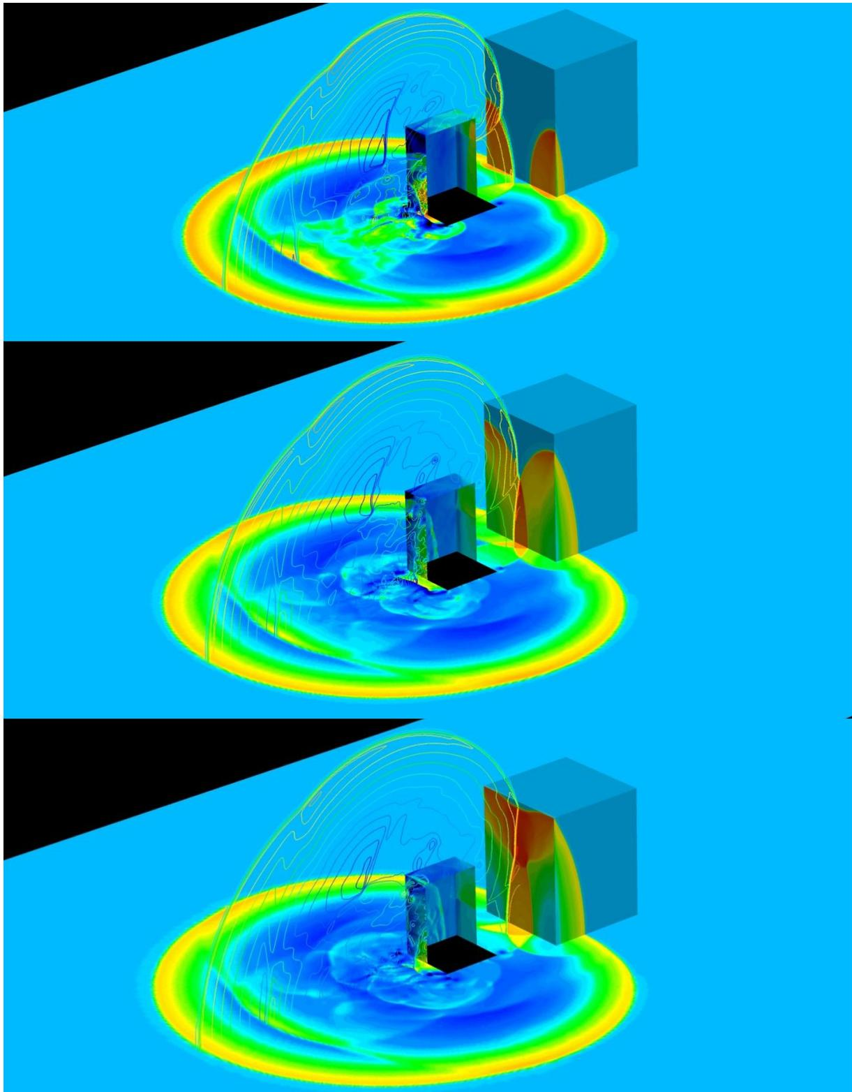
Figure 12. Time sequence with increment of 0.057 scaled time (from top to bottom) showing waves merging on the front wall of the large building
