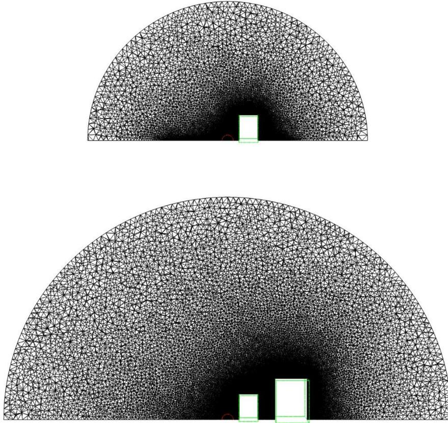
**Figure 4. Single mesh, one-building case (above), two-building case (below)**
