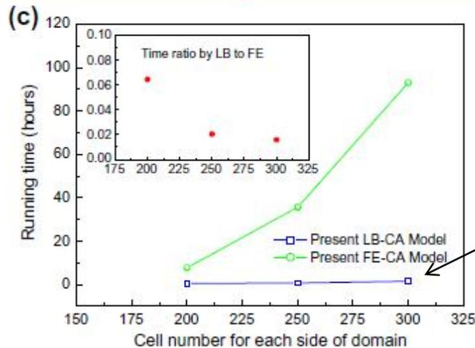
When fluid flow around solidifying dendrites is considered, lattice Boltzmann method is faster than alternatives
