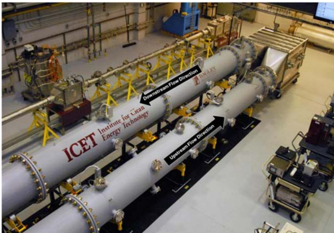
Figure 3. Photo of the MSU large scale HEPA filter test stand equipped with a housing capable of testing two 2000 cfm radial flow HEPA filters.
