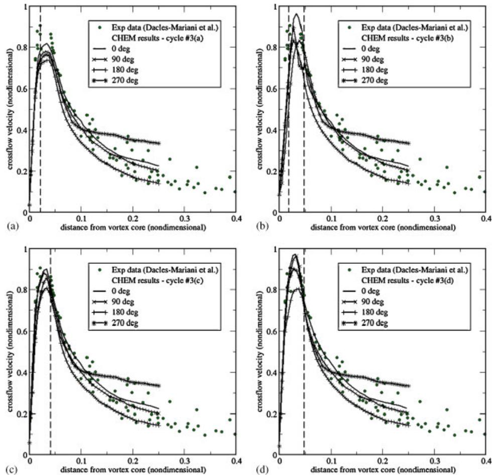
Figure 17. Extracted non-dimensional crossflow velocity for wing in wind tunnel along rays emanating from vortex core in plane at  $x/c = 1.4$ : (a) cycle #3(a) core refinement only; (b) cycle #3(b) refinement near extent; (c) cycle #3(c) refinement inside extent; and (d) cycle #3(d) refinement inside and near extent.
