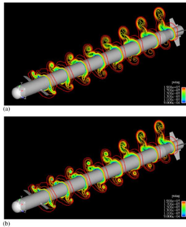
Figure 20. Stagnation pressure contours computed for missile spinning at 60 Hz. Again, the vortices are more persistent on the refined mesh than on the baseline mesh: (a) baseline mesh and (b) refined mesh (cycle 1).
