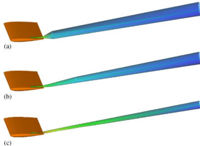
Figure 14. Vortex extent surfaces extracted from flow solutions. Note that the radius of the vortex extent decreases with refinement: (a) wingtip vortex extracted from baseline mesh; (b) wingtip vortex extracted from mesh after first refinement (cycle #1); and (c) wingtip vortex extracted from mesh after second refinement (cycle #2).
