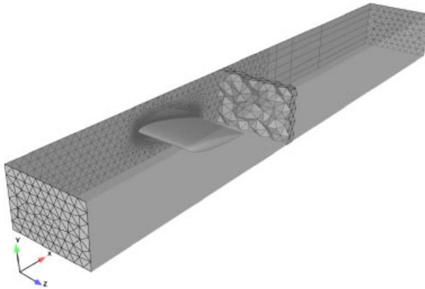
Figure 8. Computational domain employed for wing-wind tunnel computation [13]. The crinkle-cut section illustrates where comparisons are made with experimental data.
