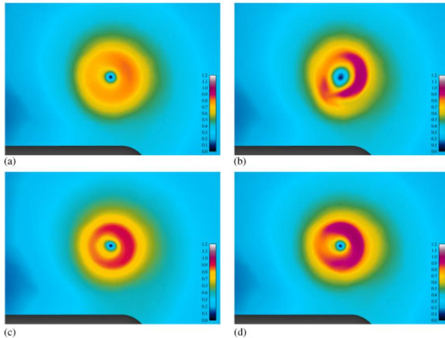
Figure 16. Non-dimensional crossflow velocity in cutting plane at  $x/c=1.4$  for wing in wind tunnel: (a) cycle #3(a) core refinement only; (b) cycle #3(b) refinement near extent; (c) cycle #3(c) refinement inside extent; and (d) cycle #3(d) refinement inside and near extent.
