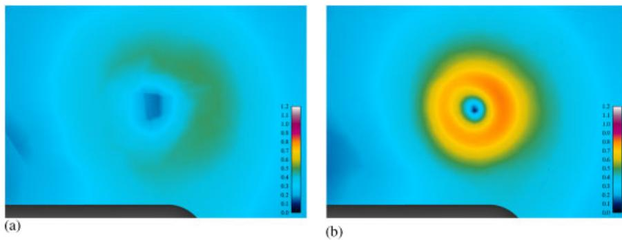
Figure 12. Non-dimensional crossflow velocity in cutting plane at  $x/c = 1.4$  for wing in wind tunnel: (a) cycle #1 and (b) cycle #2.
