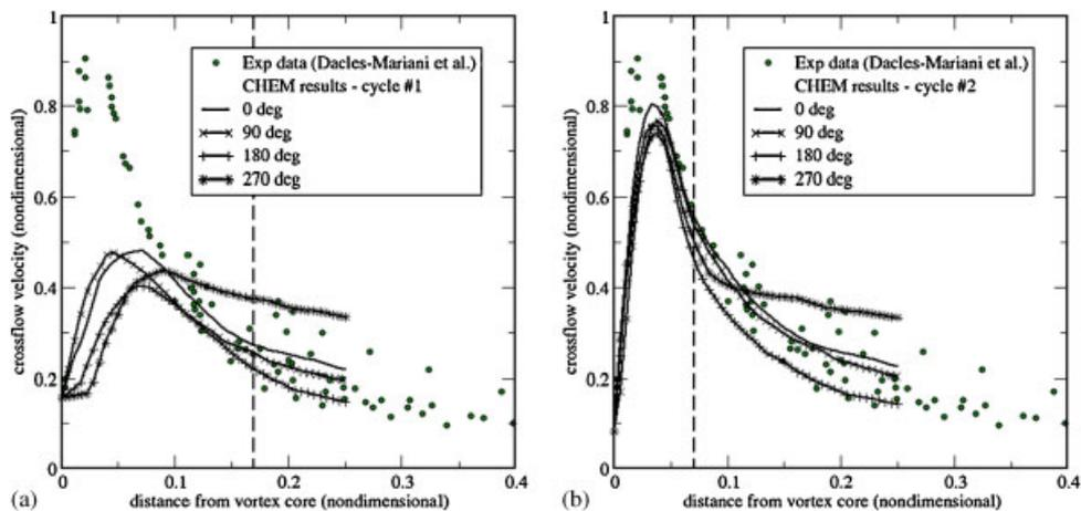
Figure 13. Extracted non-dimensional crossflow velocity along rays emanating from vortex core in plane at  $x/c = 1.4$ : (a) cycle #1 and (b) cycle #2.
