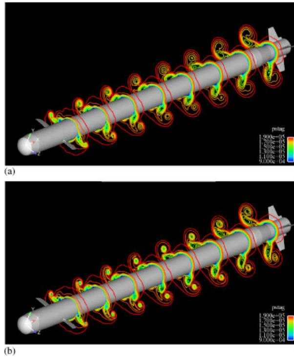
Figure 19. Stagnation pressure contours computed for missile spinning at 30 Hz. Note that the vortices predicted on the baseline mesh are diffused much more rapidly in comparison to those computed on the refined mesh: (a) baseline mesh and (b) refined mesh (cycle 1).
