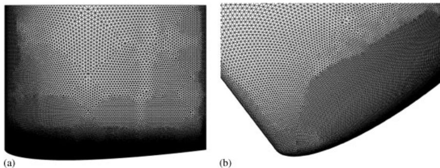
Figure 9. Wing surface mesh: (a) top view and (b) surface mesh near wing tip.
