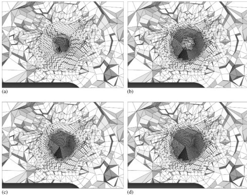
Figure 15. Mesh refinement in cutting plane at  $x/c=1.4$  for wing in wind tunnel: (a) cycle #3(a) core refinement only; (b) cycle #3(b) refinement near extent; (c) cycle #3(c) refinement inside extent; and (d) cycle #3(d) refinement inside and near extent.
