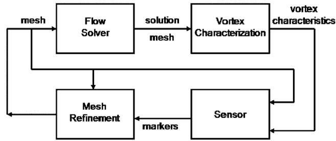
Figure 1. Schematic of adaptive mesh refinement process.
