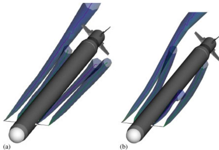
Figure 18. Extent surfaces extracted from baseline mesh solutions for missile spinning at 30 and 60 Hz: (a) baseline mesh 30 Hz and (b) baseline mesh 60 Hz.
