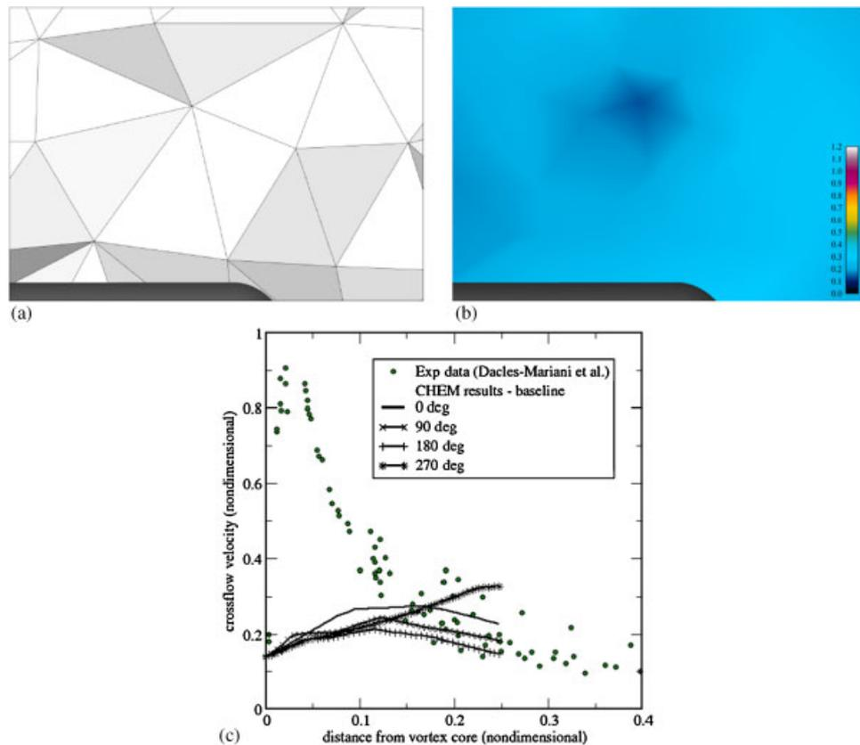
Figure 10. Cutting plane in baseline at  $x/c=1.4$  for wing in wind tunnel: (a) baseline mesh; (b) non-dimensional crossflow velocity; and (c) comparison with experimental data.
