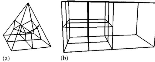
Figure 7. General elements can be created when refinement is applied to a cell with a four-valence node (left) or when a refined cell is a neighbor to an unrefined cell (right): (a) refined pyramid and (b) refined/unrefined cell neighbors.
