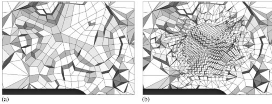
Figure 11. Mesh refinement in cutting plane at  $x/c = 1.4$  for wing in wind tunnel: (a) cycle #1 and (b) cycle #2.
