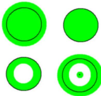
Figure 3. The circle represents vortex extent. The dot in the middle is the core line. The shaded areas show possible regions that can be marked. From left to right, top to bottom: inside extent+near extent, inside extent, inside extent–core, and near extent+near core.
