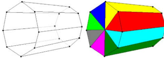
Figure 4. The extent surface is described by lofting between two closed curves on planes perpendicular to the vortex axis (left). This region is decomposed into wedges to determine if a node is inside the extent surface (right).
