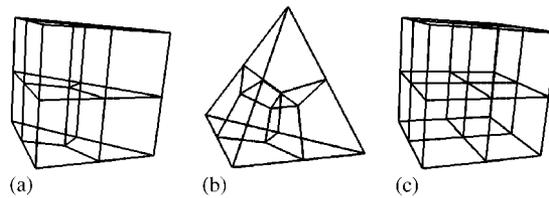
Figure 6. Canonical subdivisions for face-based isotropic refinement: (a) refined prism; (b) refined tetrahedron; and (c) refined hexahedron.
