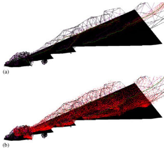
Figure 5. The sensor module can mark nodes near the core line, near the extent surface, and inside the extent surface: (a) nodes near core line marked for refinement and (b) nodes near extent surface marked for refinement.
