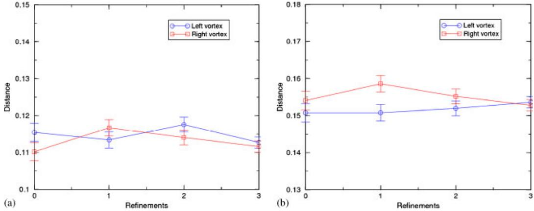
Figure 31. Mesh convergence of secondary flows in cross-section  $dd'$  (local edge length=0.007)—planar model: variation of (a) top vortex pair positions and (b) bottom vortex pair positions.
