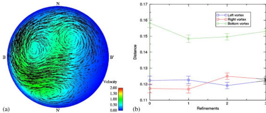
Figure 32. Mesh convergence of secondary flows in the cross-section  $dd'$ —non-planar model: (a) vortices in cross-section  $dd'$  (cross-flow velocity vectors on a cutting plane colored by velocity magnitude) and (b) variation of vortex position (local edge length=0.007).
