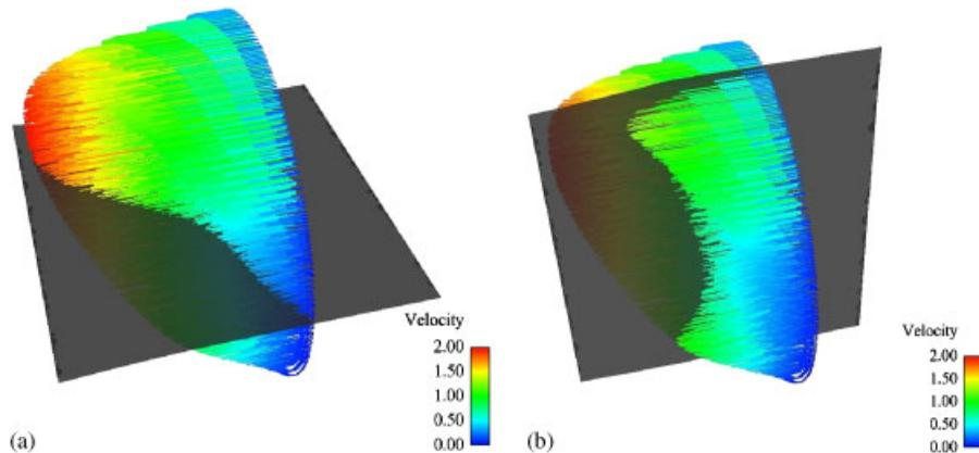
Figure 9. Three-dimensional surface plots of axial velocity profiles at  $aa'$  showing orientation of bifurcation plane and the plane normal to the bifurcation plane. Intersection of velocity profile with (a) bifurcation plane and (b) plane normal to bifurcation plane.
