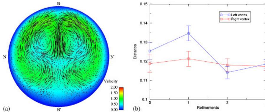
Figure 27. Mesh convergence of secondary flows in cross-section  $cc'$ —planar model: (a) vortices in cross-section  $cc'$  (cross-flow velocity vectors on a cutting plane colored by velocity magnitude) and (b) variation of vortex positions (local edge length = 0.01).
