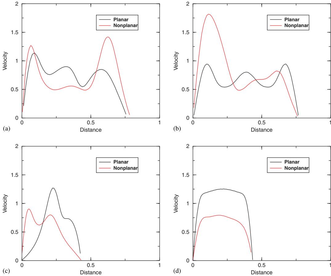
Figure 22. Comparison of the velocity distribution in third-generation branches of the planar and non-planar models: (a) in the bifurcation plane at  $cc'$ ; (b) in the plane normal to the bifurcation at  $cc'$ ; (c) in the bifurcation plane at  $dd'$ ; and (d) in the plane normal to the bifurcation at  $dd'$ .
