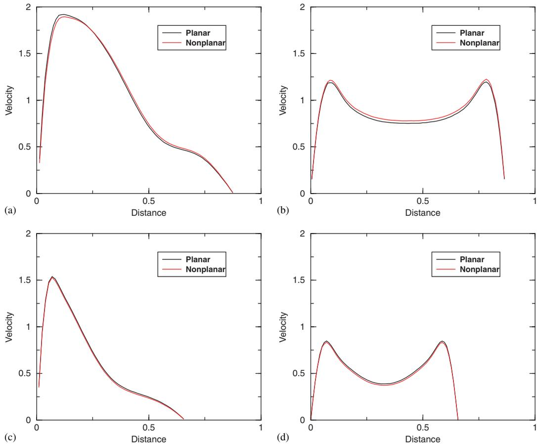
Figure 21. Comparison of the velocity distribution in second-generation branches of the planar and non-planar models: (a) in the bifurcation plane at  $aa'$ ; (b) in the plane normal to the bifurcation at  $aa'$ ; (c) in the bifurcation plane at  $bb'$ ; and (d) in the plane normal to the bifurcation at  $bb'$ .
