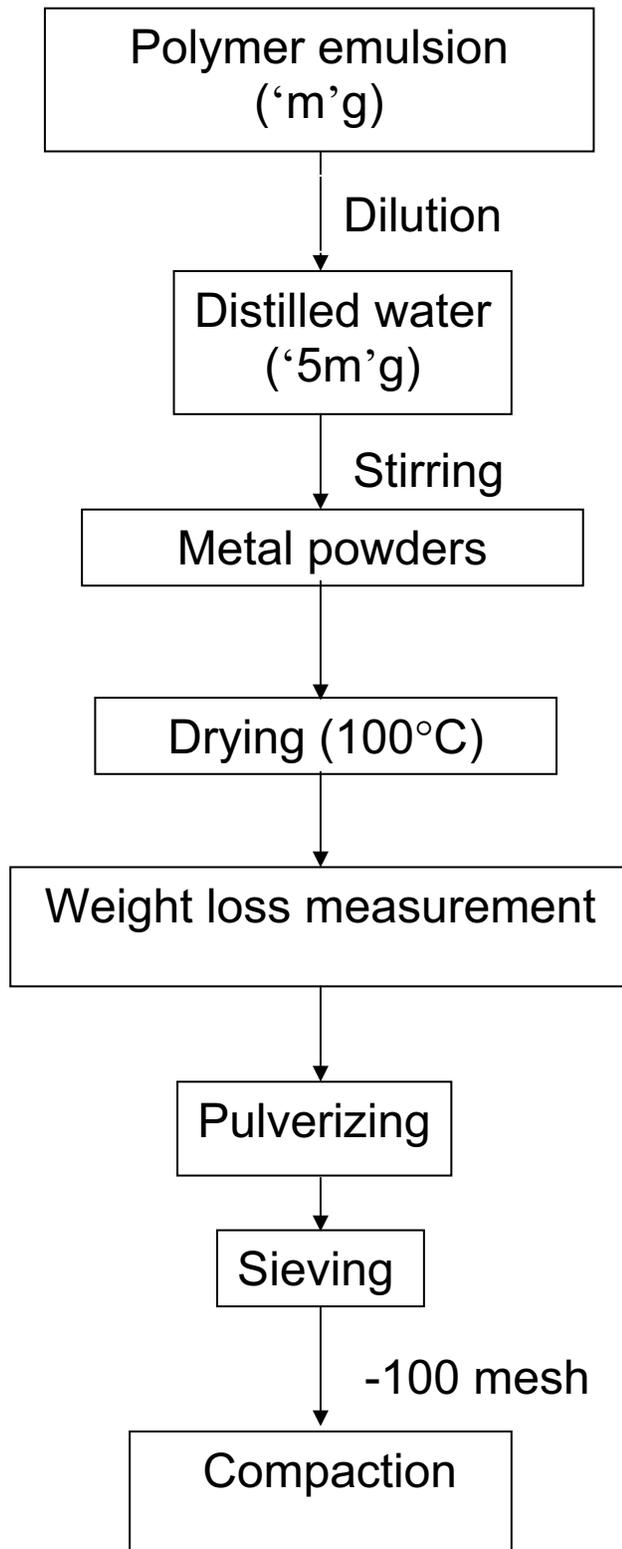
Figure 2. A brief outline of the new process developed to die compact gas atomized powders.
