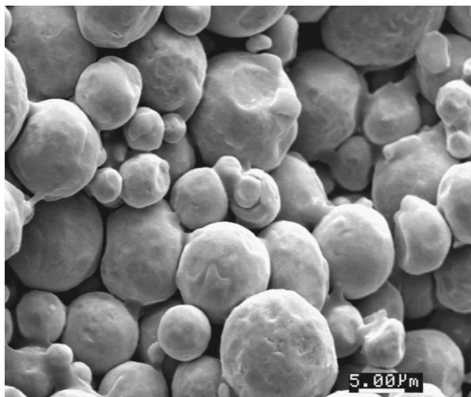
Figure 3. SEM image of fractured sample in green state showing a uniform coating of polymer on the spherical metal particles.
