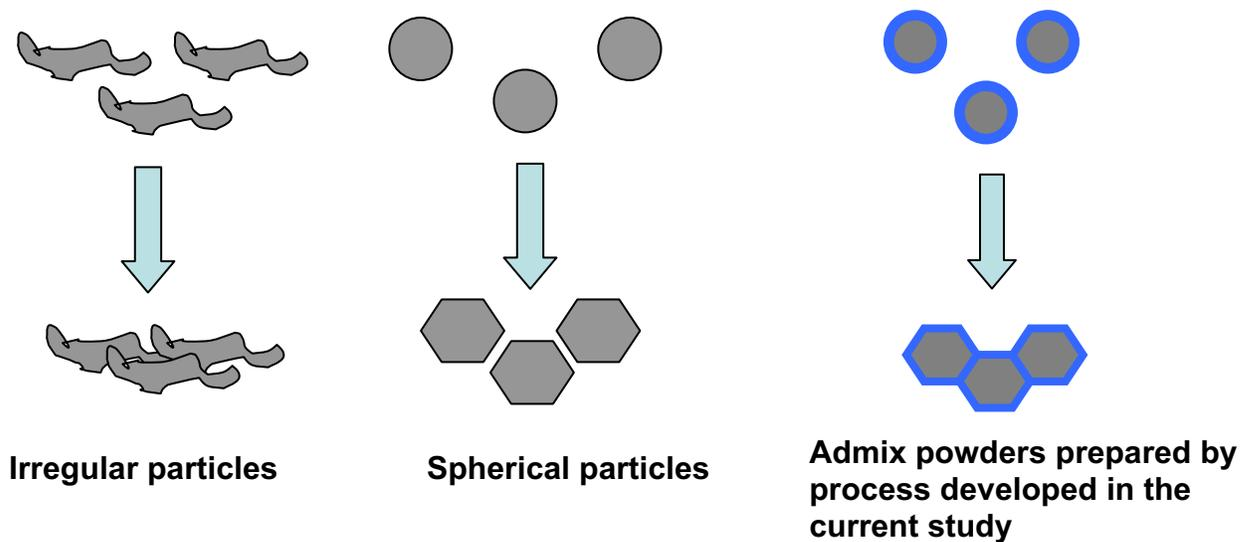
Figure 4. Schematic of the principle behind the successful compaction of admix gas atomized powders prepared from the process developed in the current study.
