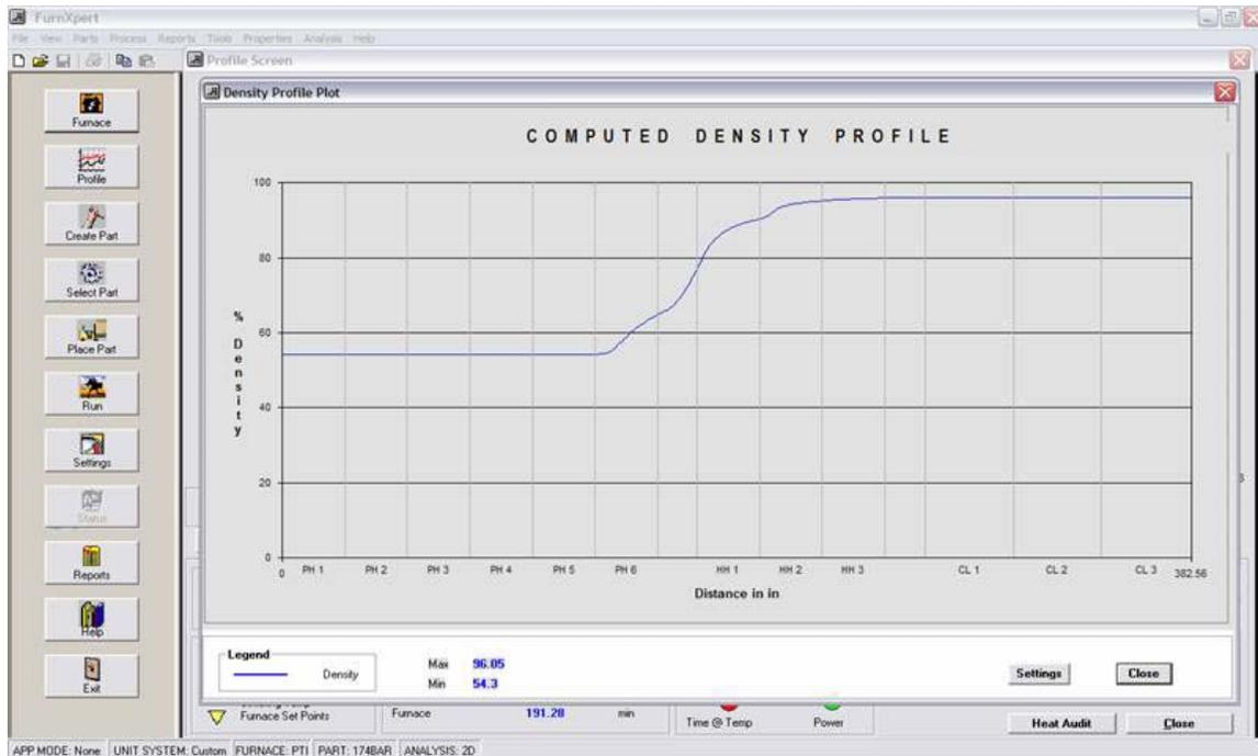
Figure 5. Example of furnace design software FURNXPRT: density evolution module
