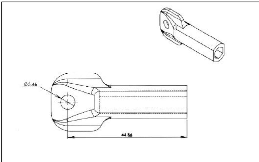
Figure 1: Drawing of the PIM component
