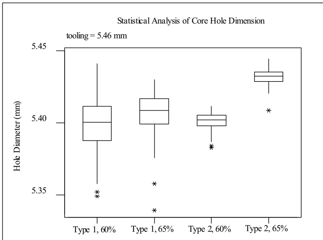
Figure 2: Variability of core hole dimension (green components)
