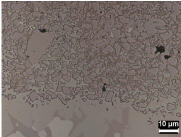
Fig 1a Interface between Ni braze B (bottom) and carbide B (top)
