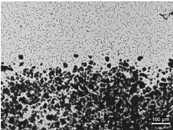
Fig 2a. Interface between Co hardface and carbide F
