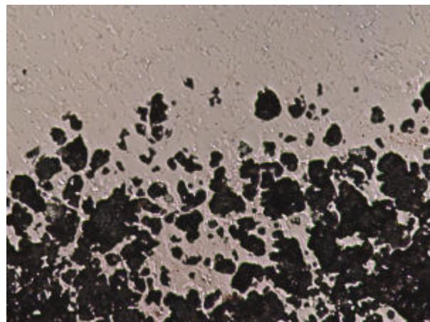
Fig 2b. Co hardface+3wt%Ti (center) and infiltrated carbide D (surrounding)
