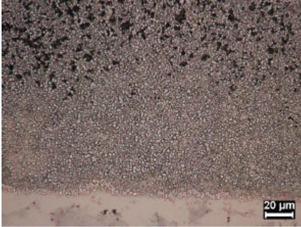
Fig 1c. Interface between Ni braze A (bottom) and carbide A (top)
