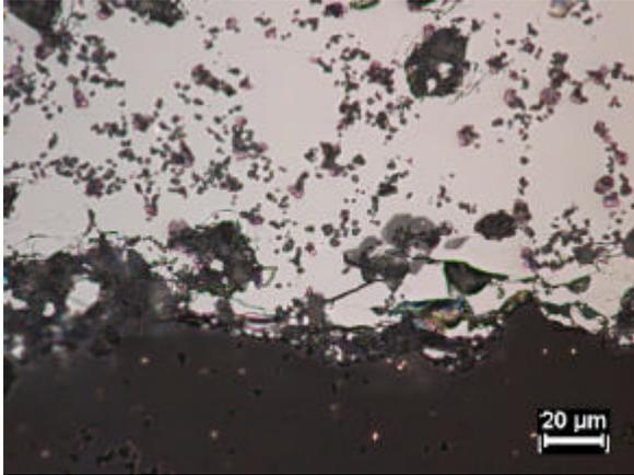
Fig 3a. Interface between Fe intermetallic (top) and uninfiltreated carbide D (bottom)
