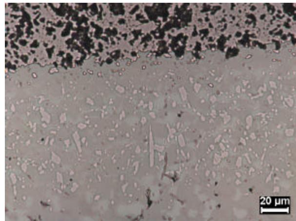
Fig 1b Interface between Ni braze B+3Wt%Ti (bottom) and carbide B (top)
