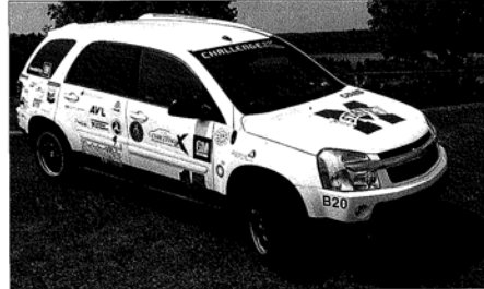
THIS CHEVROLET Equinox was re-engineered by Mississippi State University students into a hybrid vehicle powered by a diesel engine and an electric motor.
