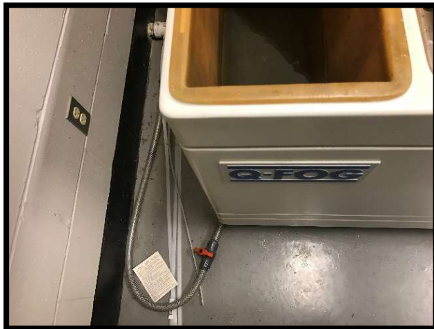
Figure 6: Salt water reservoir drainage valve (in the closed position as shown)
