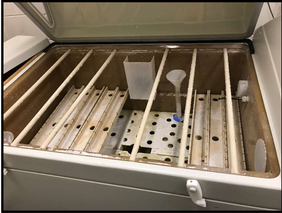
Figure 7a: Interior view of Q Fog corrosion compartment
