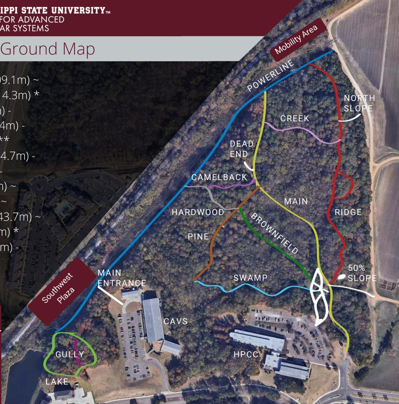
The CAVS Proving Ground is a center-wide resource for development and testing of vehicular technology, including advanced materials, unmanned aerial systems, automated vehicles, and mobility characterization.
