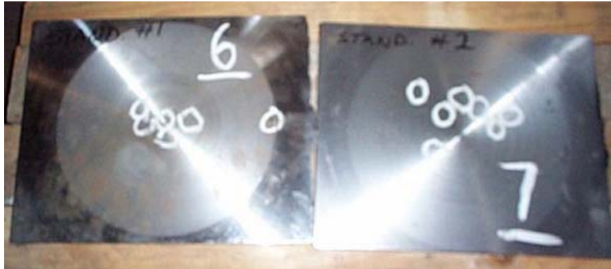
(a) Visible inclusions, as indicated by circles, on the machined surface of low-alloy steel plates (from Carlson and Beckermann, 2004).
