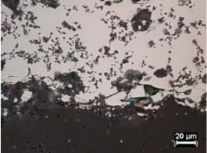
Fig 3a. Interface between Fe intermetallic (top) and uninfiltrated carbide D (bottom)
