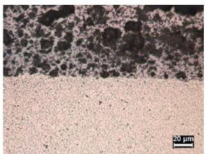
Fig 3b.Interface between Fe intermetallic +3wt%Ti (top) and infiltrated carbide D (bottom)
