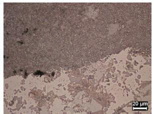
Fig 1d. Interface between Ni braze A +3wt%Ti (bottom) and carbide C (top)
