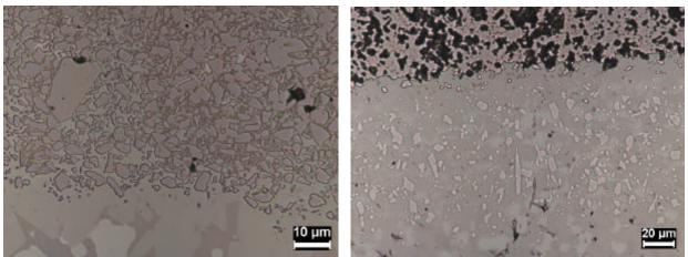
Fig 1a Interface between Ni braze B (bottom) and carbide B (top)
