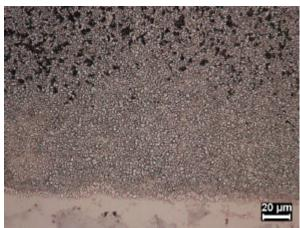
Fig 1c. Interface between Ni braze A (bottom) and carbide A (top)
