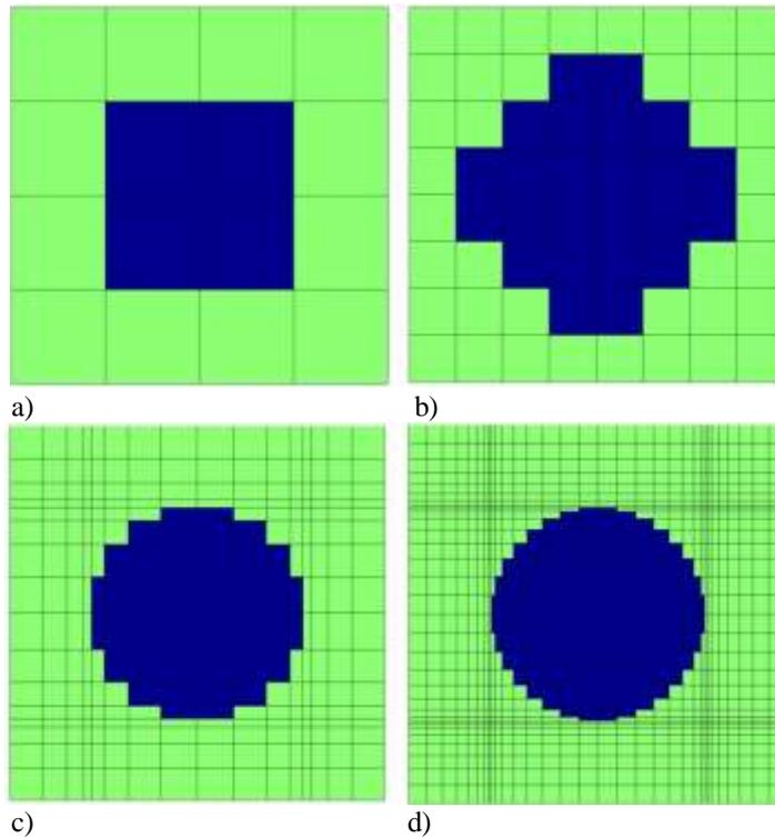
Figure 5. Four different RUC architectures comprised of a) 16, b) 64, c) 256 and d) 1024 subcells used in multiscale analyses where blue indicates a fiber subcell and green indicates a matrix subcell.
