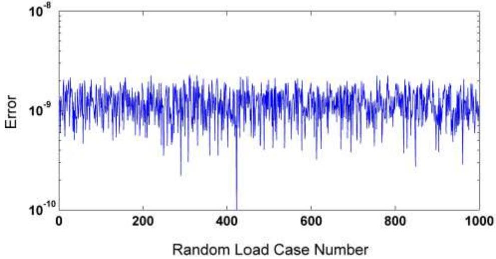
Figure 3. Error between the exact model and reduced model for each validation load case.
