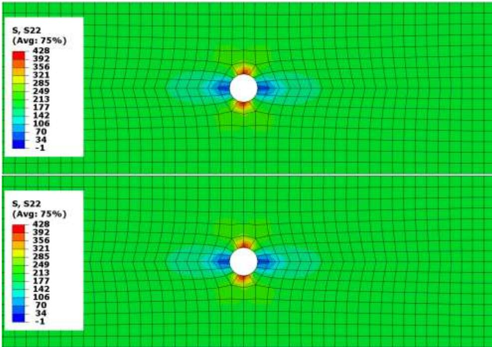
Figure 6. Comparison of the stress field in the direction of the applied loading in the vicinity of the hole where the exact (top) and order-reduced (bottom) HFGMC relationships were implemented at the microscale for a 1024 subcell RUC. All stresses are reported in units of *MPa*.
