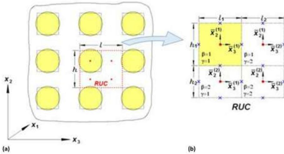
Figure 1. a) Representation of a unidirectional composite with fibers aligned in the  $x_1$ -direction and b) RUC representation of the unidirectional composite. Figure from [2].
