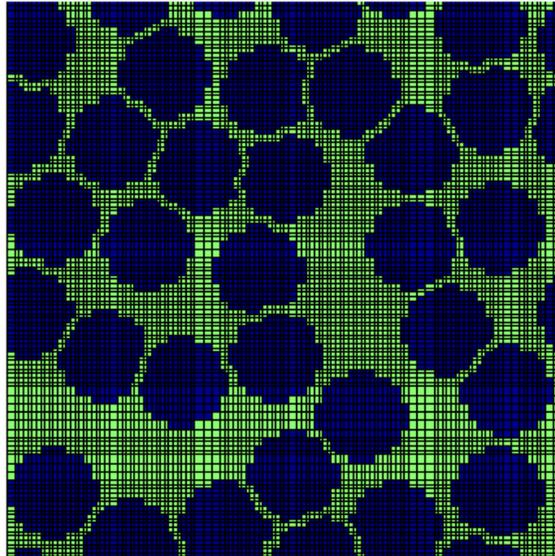
Figure 2. RUC where blue indicates a fiber subcell and green indicates a matrix subcell.
