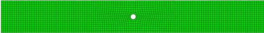
Figure 4. FE mesh of a unidirectional open-hole tensile composite specimen.
