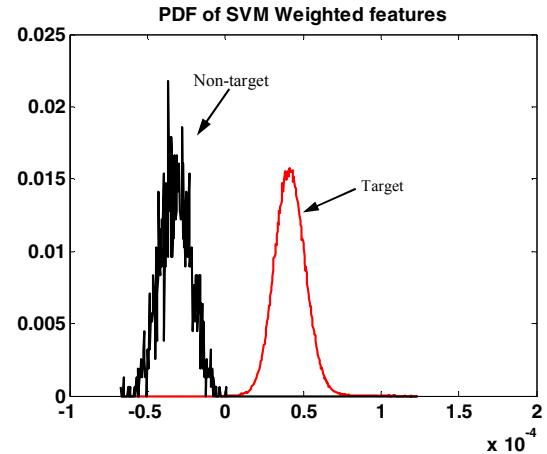
Figure 4. PDF of L-SVM statistic  $z$  for Experiment 4 (SNR = -10 dB).
