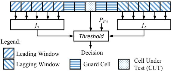
Figure 1. CFAR Processor Architecture.
