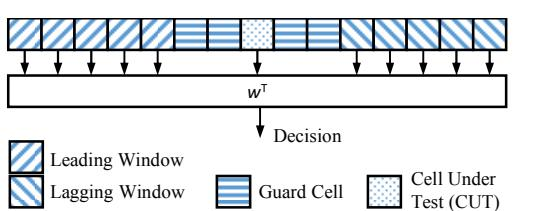
Figure 2. L-SVM Processor Architecture.
