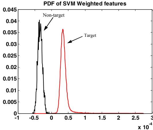
Figure 3. PDF of SVM statistic  $z$  for Experiment 1 (SNR = 5 dB).
