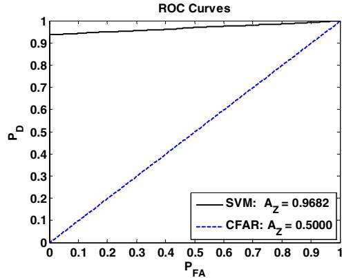
Figure 6. ROC Curves for experiment 5 (SNR = -25 dB).
