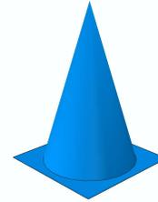
Figure 2. Geometry of the conical impactor used in the simulations. The sharp nose is used to generate a ductile failure mode of the tank car during the impact.
