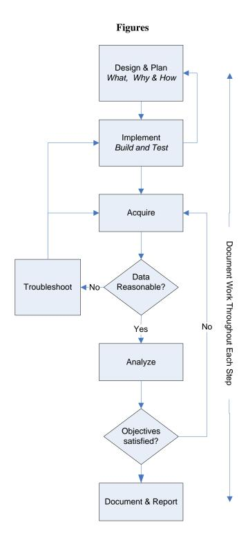
Figure 1 Experimentation planning flowchart (Fig. 7 in Ref. 2)
