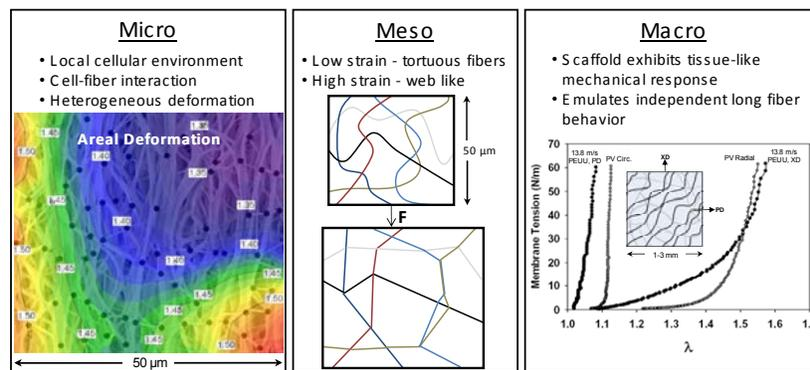
**Fig 3.** Despite exhibiting gross tissue-like mechanical response at the macro scale, the scaffold exhibits unique micro and meso mechanical behaviors. For instance, at the micro-scale a heterogeneous deformation response is observed. In addition, fibers in the unstrained configuration exhibit an undulated or tortuous morphology which transitions to a highly interconnected web-like architecture at finite strains [2].
