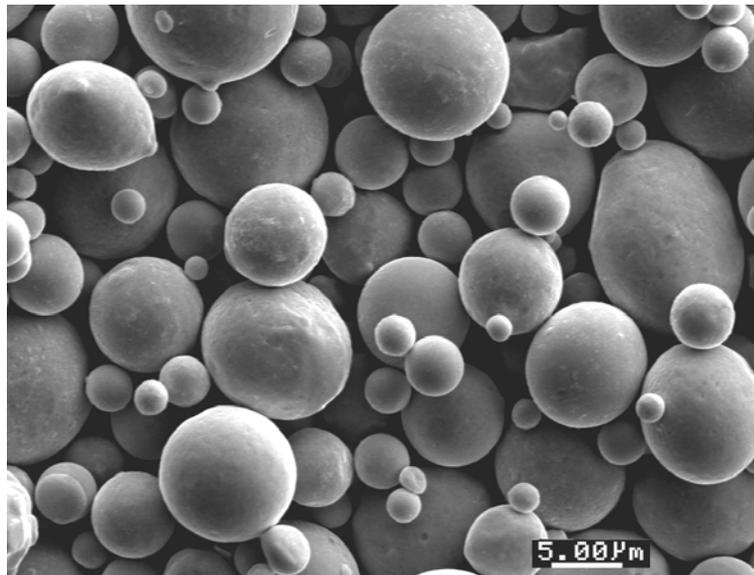
Figure 1: Scanning electron micrograph of as-received gas atomized 316L stainless steel powder.
