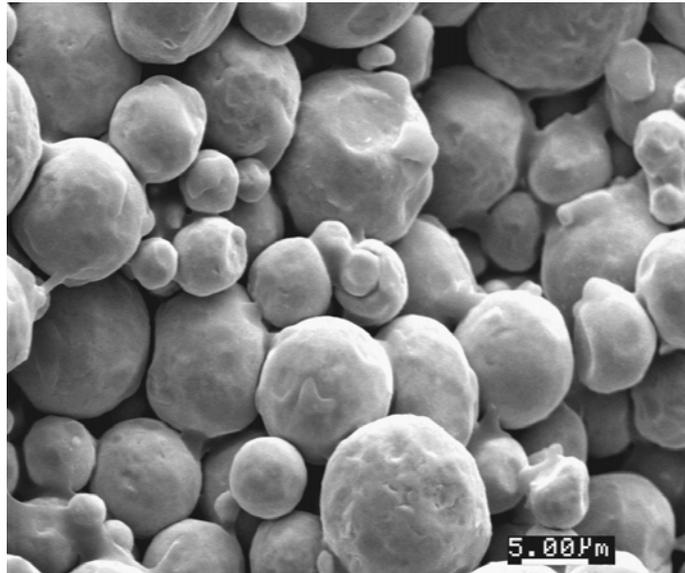
Figure 3. SEM image of fractured sample in green state showing a uniform coating of polymer on the spherical metal particles.
