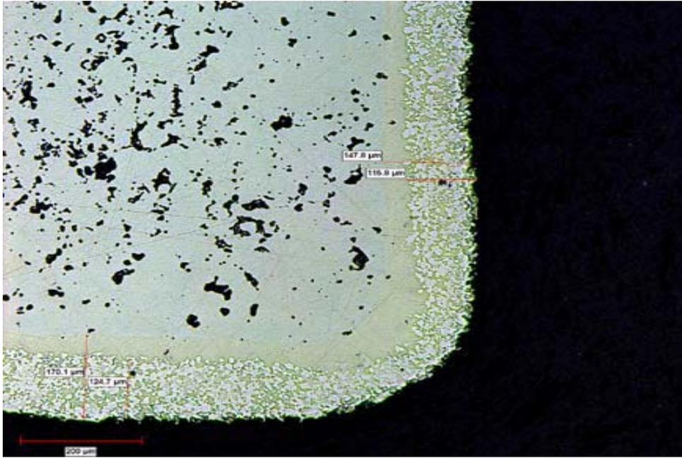
Figure 9. Sprayed two-layer coating, vacuum sintered at  $1160^{\circ}C$ , showing corner rounding.
