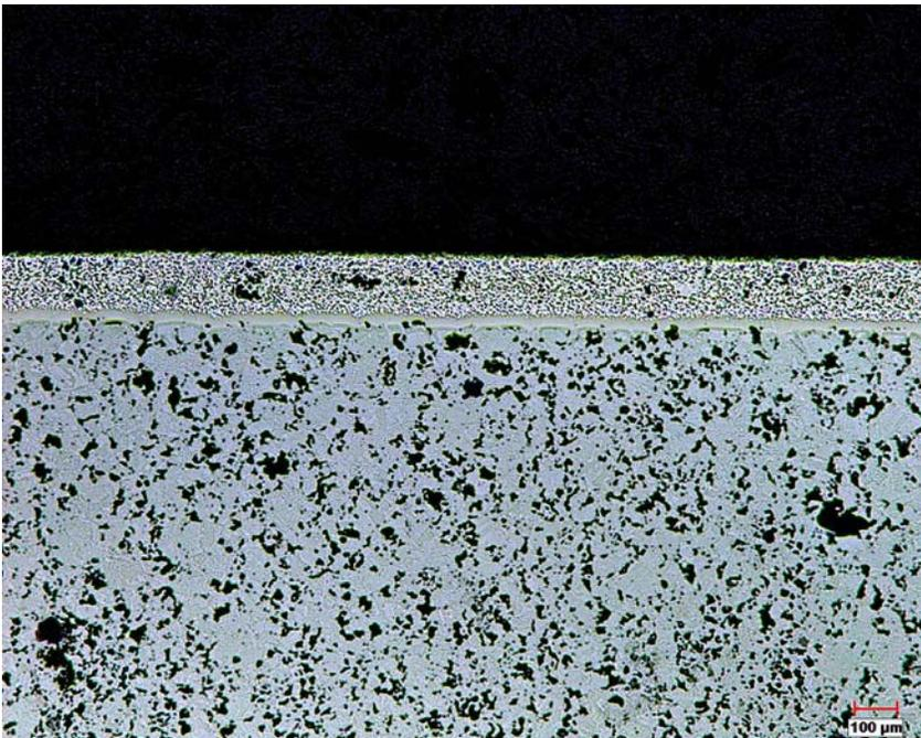
Figure 3. BNi-5- Cr<sub>3</sub>C<sub>2</sub> coating on P/M steel (bottom) with braze/carbide ratio of ~0.8. Coating is bonded, but steel is not infiltrated.
