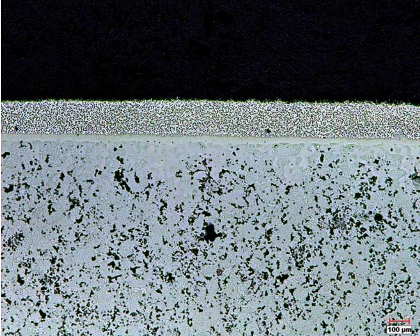
Figure 4. BNi-5- Cr<sub>3</sub>C<sub>2</sub> coating on P/M steel (bottom) with braze/carbide ratio of ~1.2. The pores in the steel adjacent to the coating is partially infiltrated.
