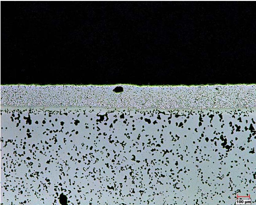
Figure 7. BNi-9 - Cr<sub>3</sub>C<sub>2</sub> coating on P/M steel (bottom) with a braze/carbide ratio of ~1.0. Spherodization and growth of pores in the P/M steel near the coating.
