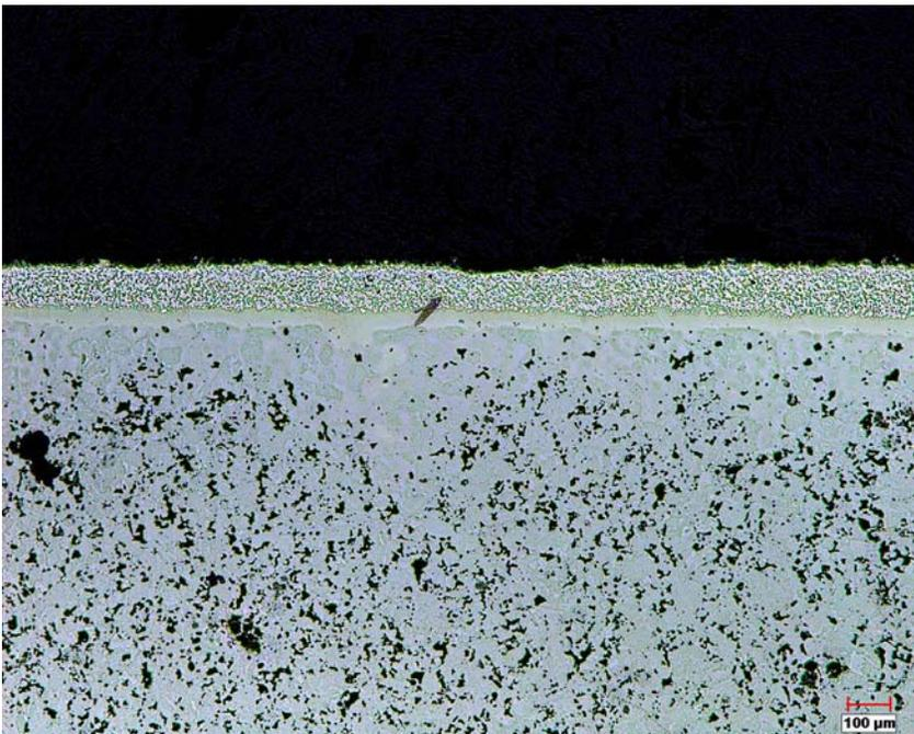
Figure 5. BNi-5- Cr<sub>3</sub>C<sub>2</sub> coating on P/M steel (bottom) with braze/carbide ratio of ~1.5. The pores in the steel adjacent to the coating is partially infiltrated, and the braze layer between the steel and coating is thicker than observed in Figures 3 and 4.
