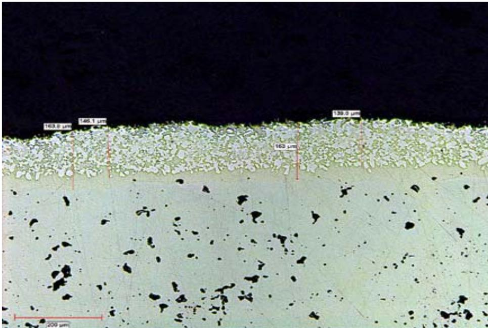
Figure 10. Sintered EPD carbide coating with sprayed braze coating, vacuum sintered at  $1160^{\circ}C$ .
