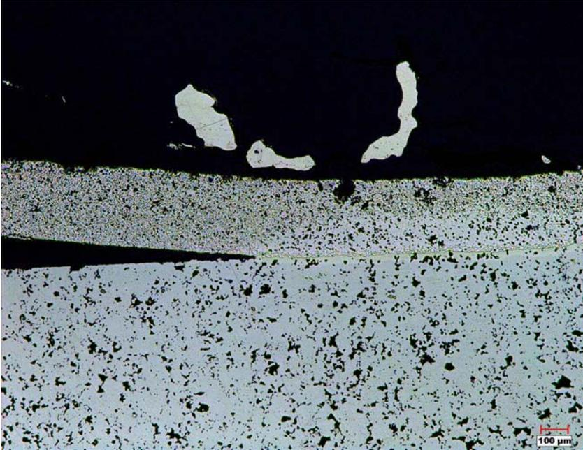
Figure 2. BNi-4- Cr<sub>3</sub>C<sub>2</sub> coating on P/M steel with a braze/carbide ratio of ~0.8. Material on top is braze alloy that did not infiltrate the carbide layer (middle), which is still porous.
