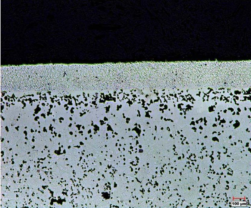
Figure 8. BNi-9 – Cr<sub>3</sub>C<sub>2</sub> coating on P/M steel (bottom) with a braze/carbide ratio of ~1.5. Increased spheroidization and growth of pores in the P/M steel near the coating.
