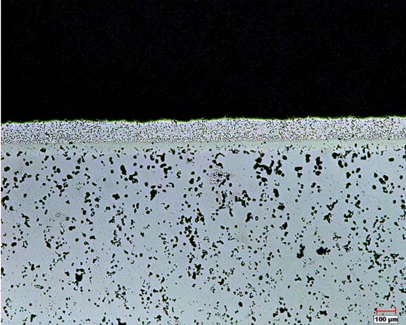
Figure 6. BNi-9 - Cr<sub>3</sub>C<sub>2</sub> coating on P/M steel (bottom) with a braze/carbide ratio of ~0.8. Slight spherodization of pores in the P/M steel near the coating.
