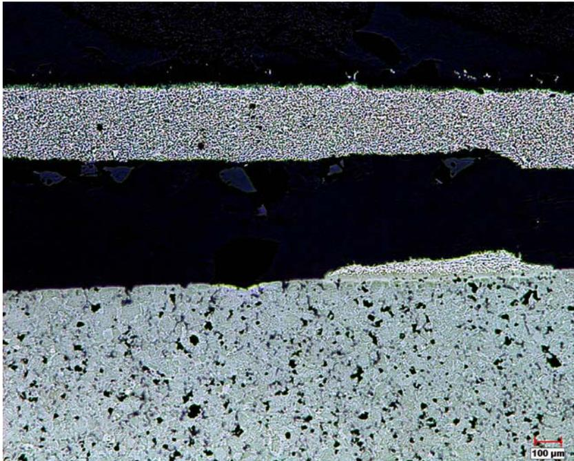
Figure 1. BNi-1a –  $\text{Cr}_3\text{C}_2$  coating on P/M steel with a braze/carbide ratio of  $\sim 1.1$ . Coating (top) is fully infiltrated, but did not bond well to steel (bottom).
