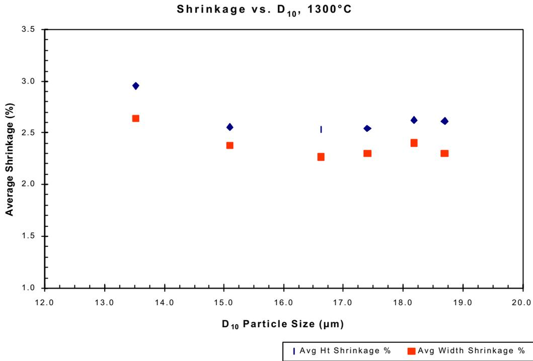
Figure 5. Shrinkage vs. D<sub>10</sub> particle size at 1300°C.
