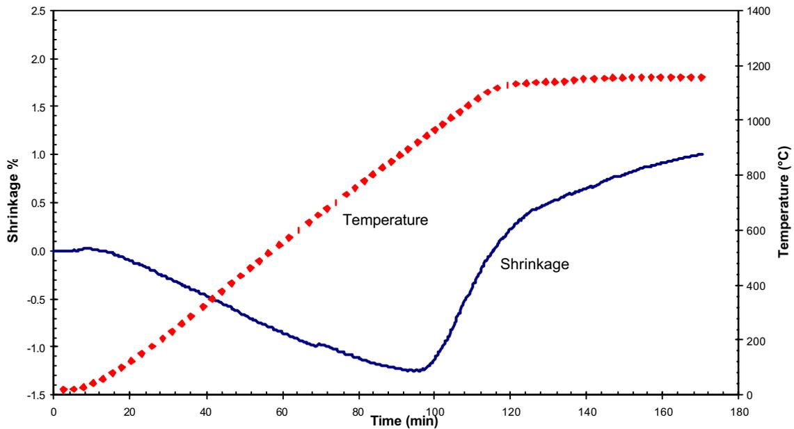
Figure 1. Dilatometry of 316L grade 1. Sample heated at 10°C/min to 1150°C for 1 h in hydrogen.
