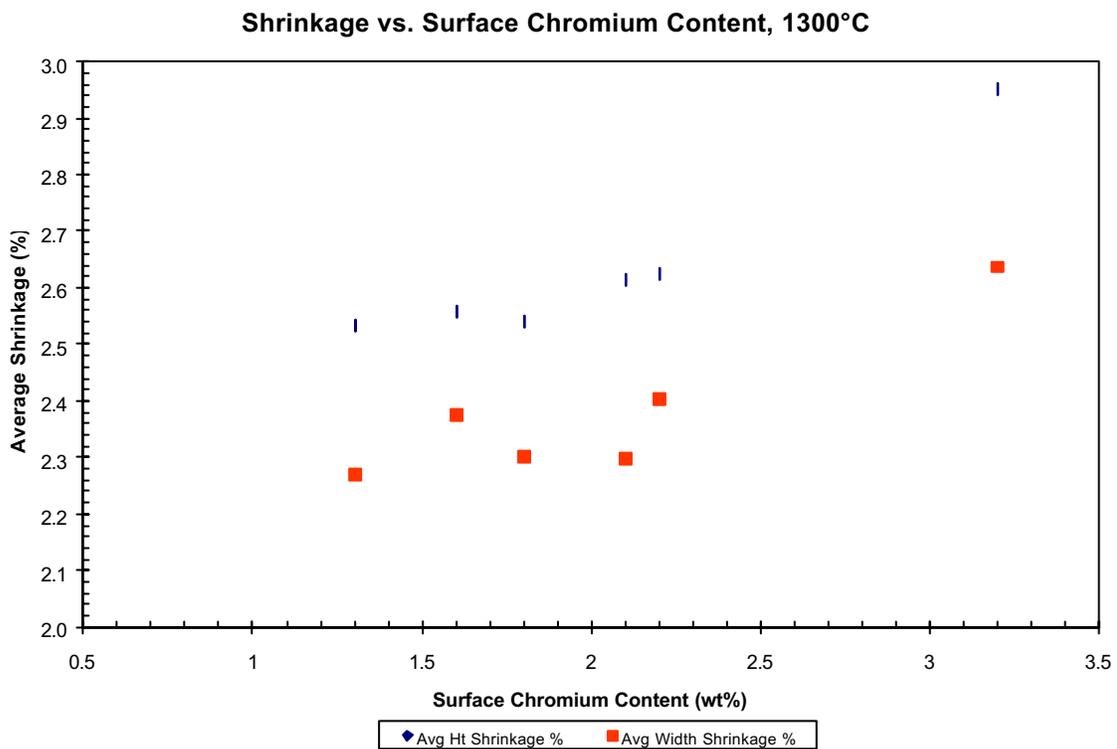
Figure 4. Shrinkage vs surface Cr content at 1300°C
