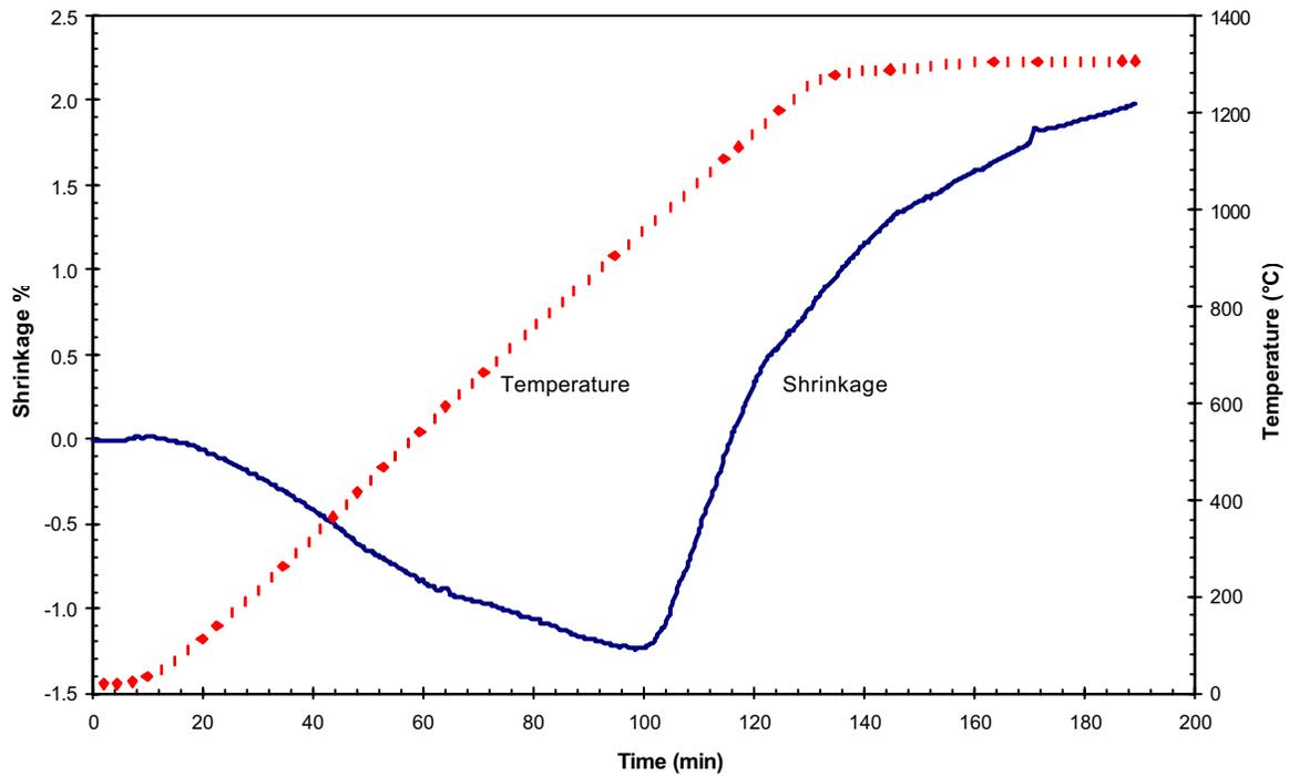
Figure 2. Dilatometry of 316L grade 1. Sample heated at 10°C/min to 1300°C for 1 h in hydrogen.
