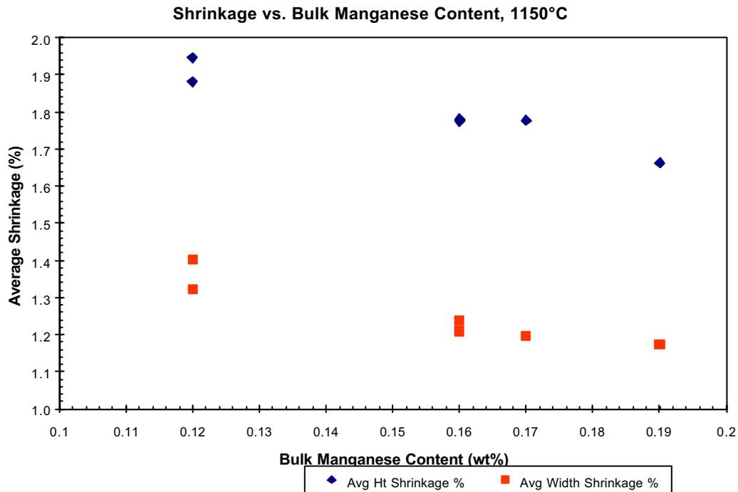
Figure 3. Shrinkage vs. bulk Mn content at 1150°C.
