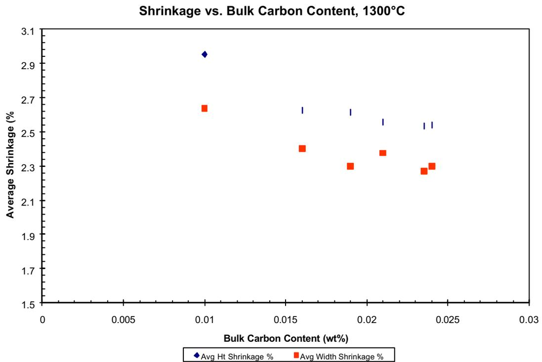
Figure 6. Shrinkage vs. bulk carbon content at 1300°C
