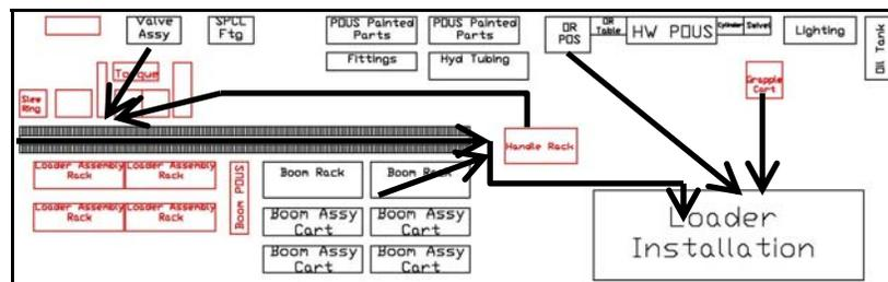
Figure 2: Current Loader Assembly Line Layout
