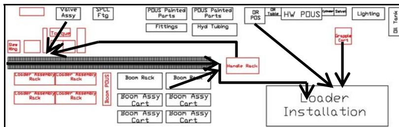
Figure 2: Current Loader Assembly Line Layout
