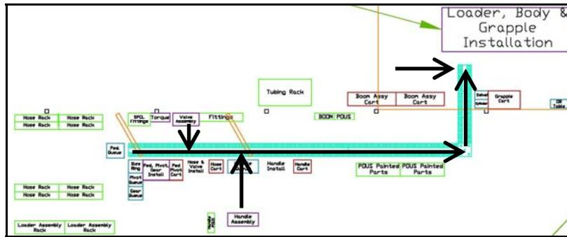
Figure 4: Proposed Loader Assembly Line Layout
