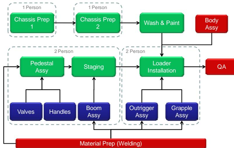
Figure 1: Loader Assembly Production Flow
