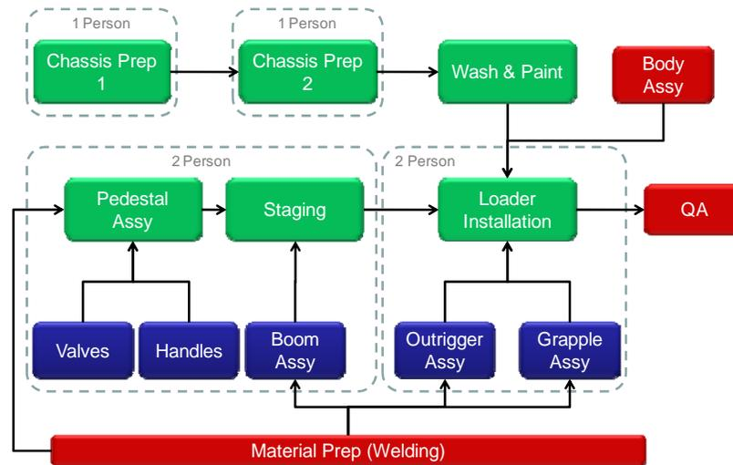
Figure 1: Loader Assembly Production Flow
