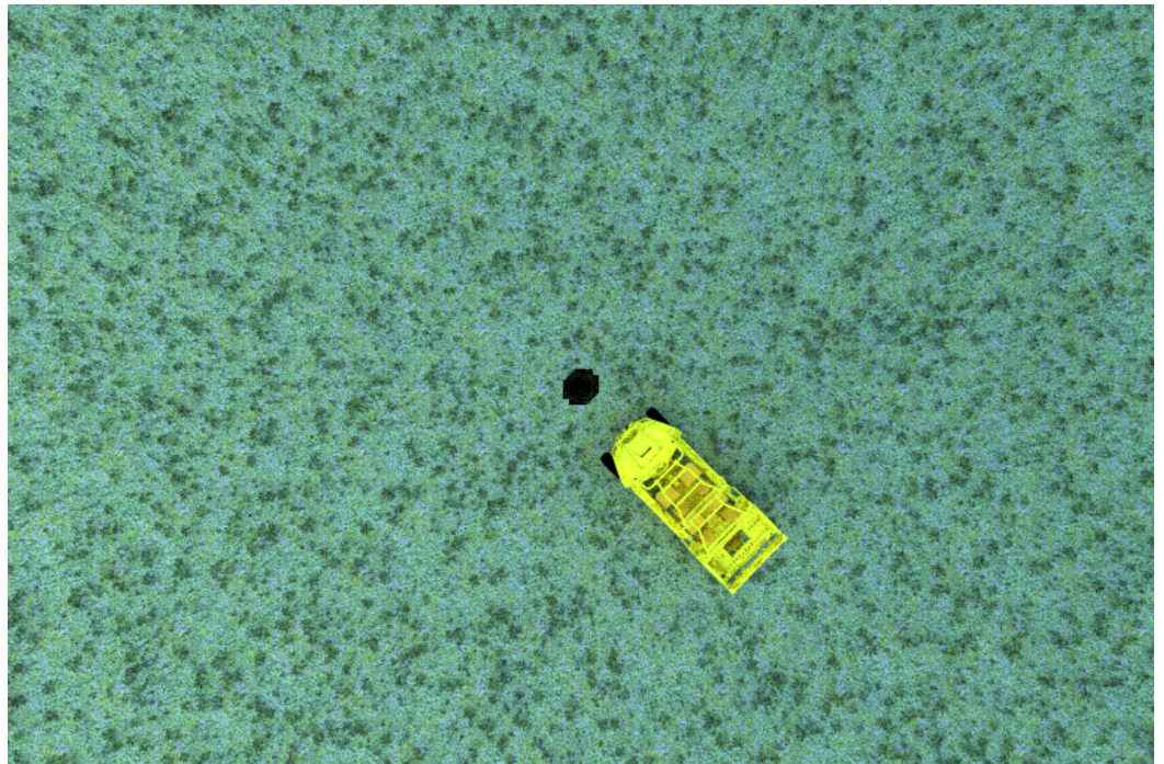
Figure 5. Rendering of the simulated scenario. The UGV moves toward the negative obstacle, a hole which is large enough to damage or immobilize the vehicle.
