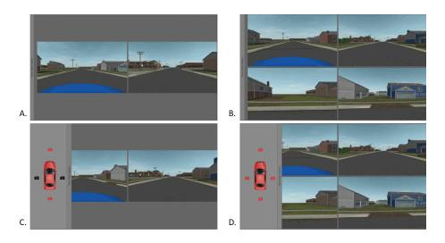
**Fig. 2.** A) Forward and rear camera on, Full Screen, B) Forward, rear, left, right camera on, Full Screen, C) Forward and rear camera on, selection slider shown, D) Forward, rear, left, right camera on, selection slider shown
