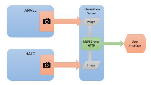
Fig. 1. The flow of video data from source to interface.
